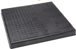
The Black Pad uses ground, recycled rubber in a co-injection process. The pad is extremely durable, resistant to ultraviolet light, and heavier than a completely plastic pad. Use 3 inch pads where local codes supersede the International code and require a pad thicker than 2".
