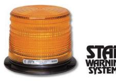
Field selectable flash pattern via internal jumper: standard quad flash or selectable double flash. Virgin Lexan, twistoff lens. Durable and lightweight polycarbonate plastic universal flange base. Completely encapsulated circuit for increased weather and shock resistance. Automatic low voltage shutdown below 9.5V DC.
