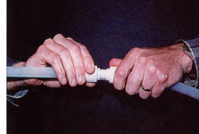
3. Slide the nut to threads and hand tighten securely onto the fitting.
